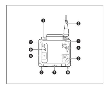
**1** Audio input connector (mini 3-pin with lock) Connects to a lavalier microphone.
