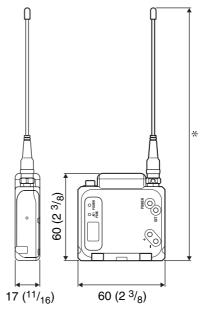
\* UC/CE L model: 214 (8 <sup>1</sup>/<sub>2</sub>) \* CE H model: 181 (7 <sup>1</sup>/<sub>4</sub>)
