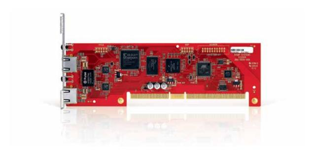
The Tesira SCM-1 is a modular digital audio networking card for use with Tesira SERVER and SERVER-IO devices. The SCM-1 allows a Tesira system to send and receive digital audio using the CobraNet® networking protocol. Each SCM-1 CobraNet card allows for interconnectivity of up to 32 x 32 channels of digital audio. Implementing the SCM-1 allows a Tesira system to share audio with Biamp Audia® and Vocia® systems as well as other devices operating on a CobraNet network.
