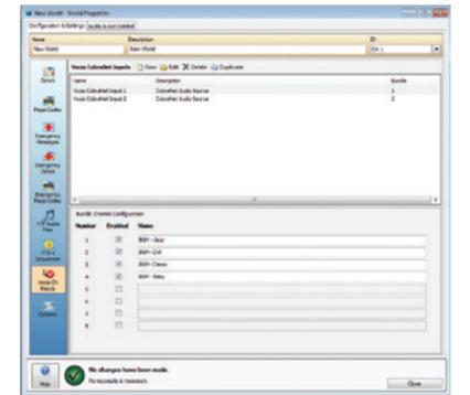
The Vocia TTS-1e Text-to-Speech server supports a windows client that is used to enter the text segments for speech conversion. The LSI-16/LSI-16e supports a browser interface for remote monitoring of emergency faults.
