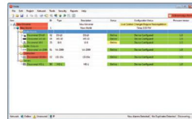
The software is designed for ease-of-use and intuitive interfacing. Most of Vocia's devices offer fixed-chain DSP parameter adjustment and live control. This screen shows the properties sheet of the VI-6 with its audio and live control settings; filters are applied to the input levels, representing one possible configuration. The filters are displayed as individual lines in the EQ filter graphic.
