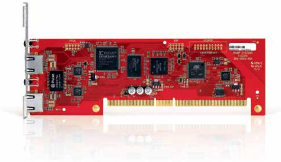
The Tesira SCM-1 is a modular digital audio networking card for use with Tesira SERVER and SERVER-IO devices. The SCM-1 allows a Tesira system to send and receive digital audio using the CobraNet® networking protocol. Each SCM-1 CobraNet card allows for interconnectivity of up to 32 x 32 channels of digital audio. Implementing the SCM-1 allows a Tesira system to share audio with Biamp Audia® and Vocia® systems as well as other devices operating on a CobraNet network.
