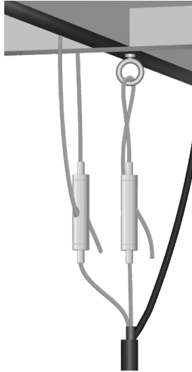
Figure 1a. Support cables can loop around structural members or through anchored hardware
