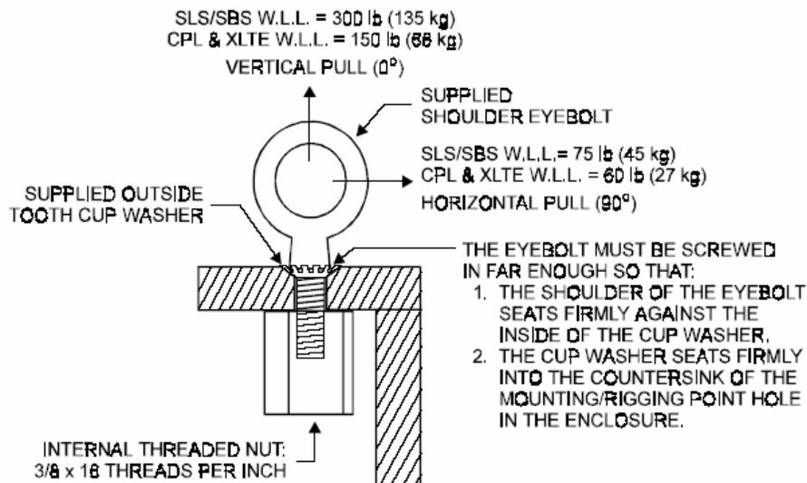
DIAGRAM: Cross-section of Mounting Rigging Point
