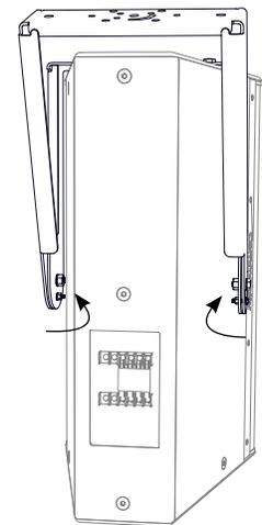
Figure 2. Fully tighten hardware to secure angle
