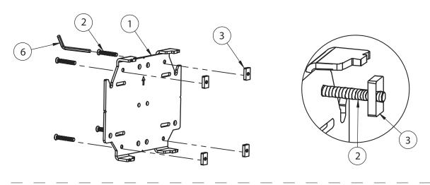
ii. Slide item 1 down the front slots of the column to the correct height and tighten items 2.
