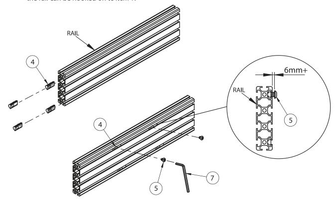
iii. Hook rail onto item 1 and fix with in place with item 5.
