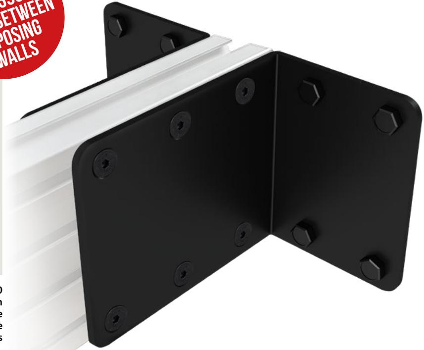
The BT8390-WFK4 is a bracket designed to fix BT8390 mounting rails between opposing walls, for the installation of menu boards and other multi-screen configurations. The plates fix the ends of the rail to the wall at a 90° angle, and are ideal for installations where the back wall is not present or is unsuitable for mounting.
