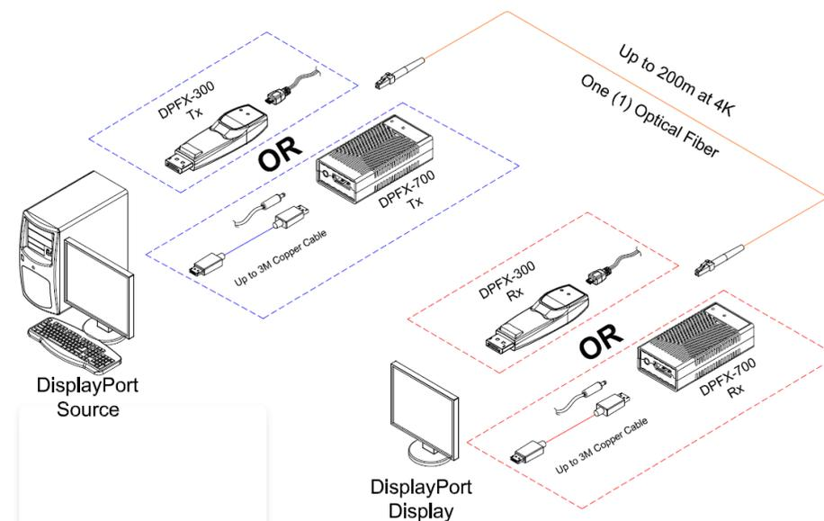
Fig Figure 3 – Connection of optical fiber
