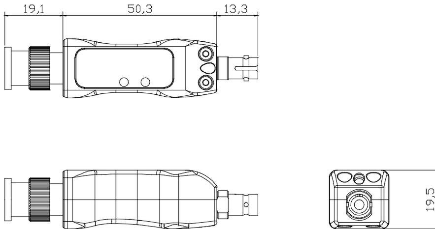
Note: The transmitter, SDIX-100-T and the receiver, SDIX-100C-R have the same mechanical dimensions.
