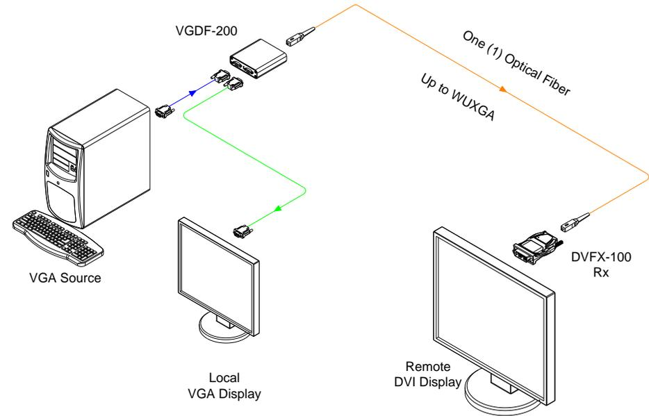
Figure 1 – Connection Diagram of VGDF-200
