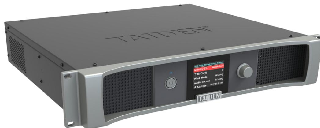
HCS-5100M/B Series Digital Infrared Transmitter adopts DQPSK digital modulation/demodulation technology to connect interpreter units to realize simultaneous interpretation, etc. Suitable for small, medium and large international conference halls or outdoor venues. Due to the high transmission frequency (1~8 MHz), it fully satisfies the user's demand for secure, confidential and interference-free meetings.
