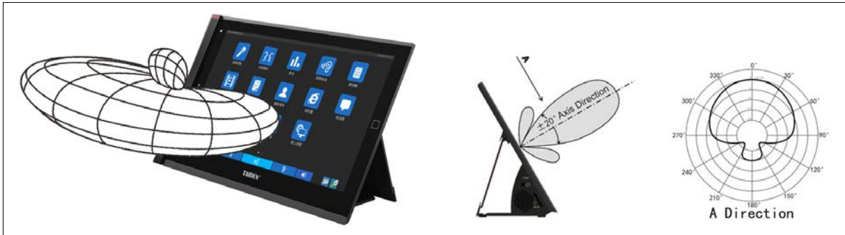
Figure 9 Polar pattern of HCS-8368A/50 Paperless Multimedia Congress Terminal
