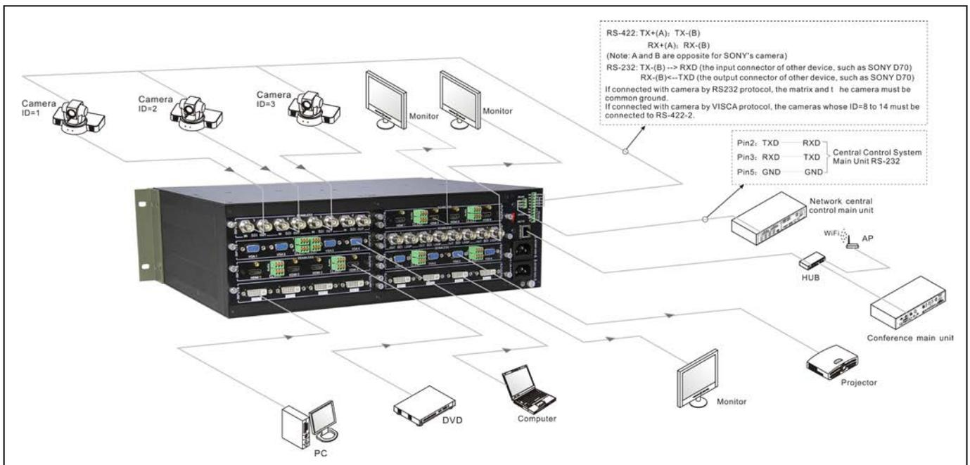
Figure 1.3 Connection for input and output devices to Mixed Card Matrix Switcher
