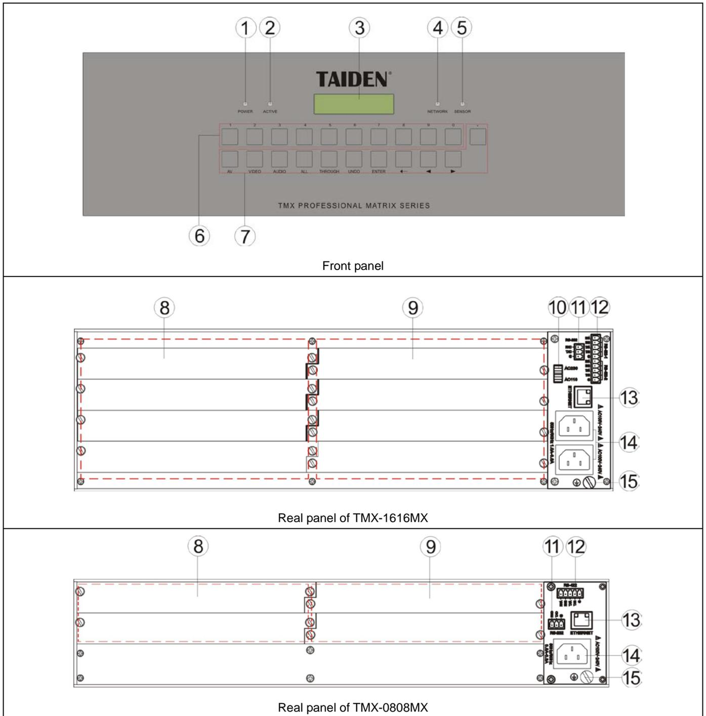
Figure 1.1 Panels of Mixed Card Matrix Switcher
