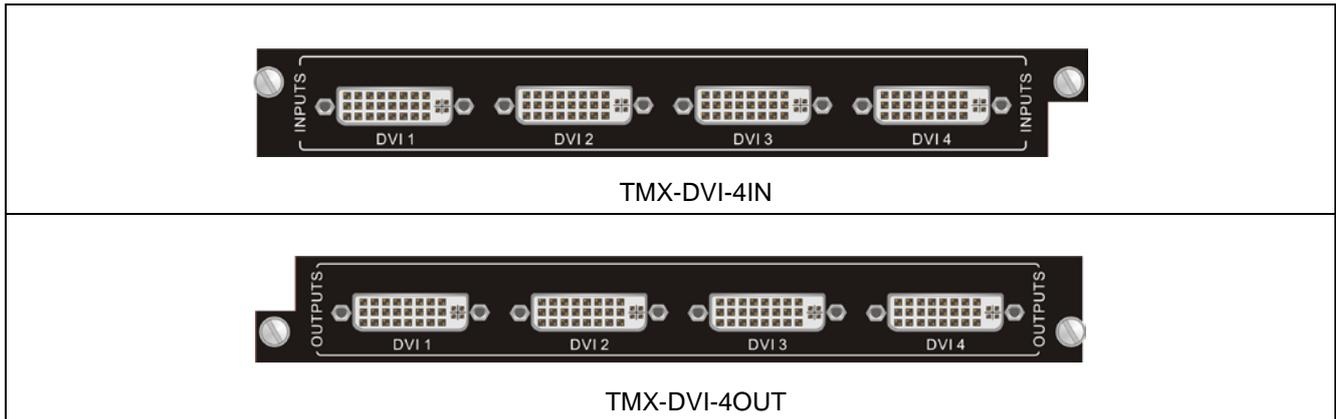
Figure 2.2 4 Channels DVI-I Input/Output Signal Card
